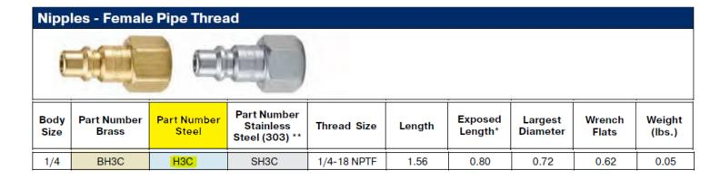
Industrial Interchange Nipples are compatible for use with 20 Series, 30 Series, Rectus 21, 23, 30 Series, Universal or E-z-mate couplers. The standard male tip of the pneumatic industry, these nipples are interchangeable with similar nipples manufactured to the same requirements.
