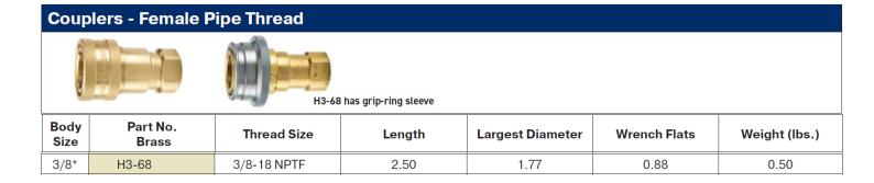
60 Series Steam couplings are brass with stainless steel locking balls and ethylene propylene seals to withstand temperatures up to 400°F/205°C
